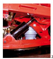
2 powerful hydraulic cylinders control the levelling of the bundler on
