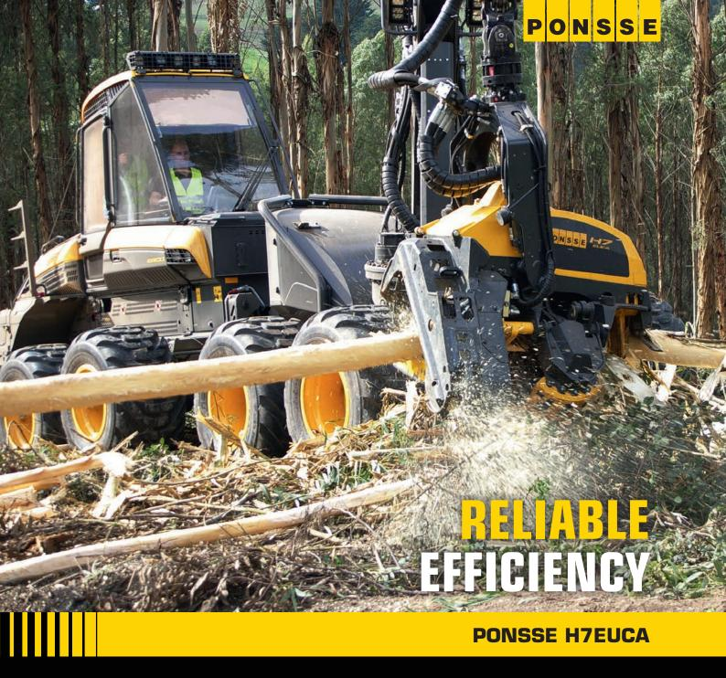
PONSSE H7euca is a new generation harvester head for debarking the trees during processing. The H7euca is based on long experience of the PONSSE harvester head family, the reliability and the excellent characteristics of the H7 harvester head and the experience of debarking requirements.
