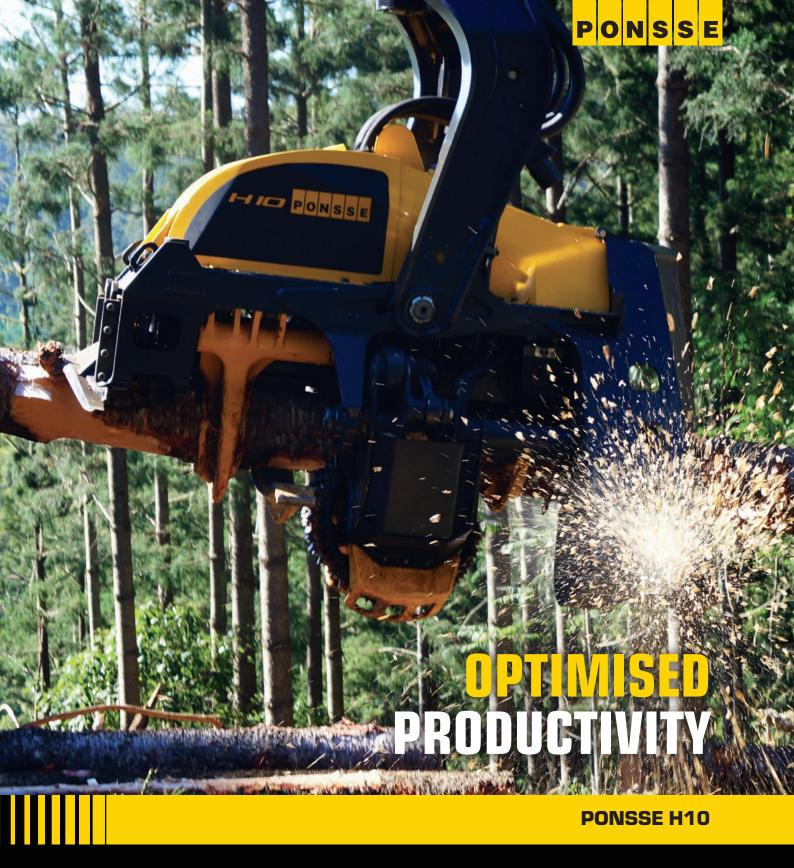
THE PONSSE H10 PROCESSING HEAD offers PONSSE quality and productivity to a new size class. The PONSSE H10 is designed and built for heavy-duty processing work in tough conditions. Robust structure, strong grip and powerful feeding guarantee high efficiency and reliability. With a flexible and widely adjustable Opti system, you are always in full control of you operations. PONSSE H10 harvester head is designed to keep you productive through the years.
